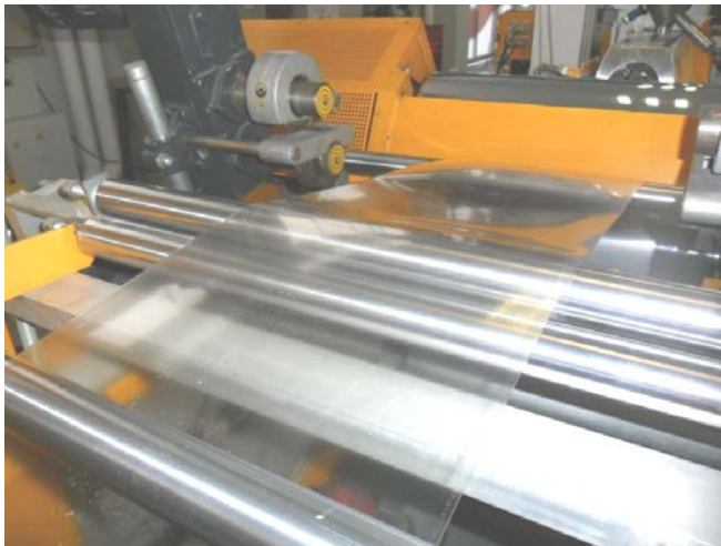
Flat film extrusion
