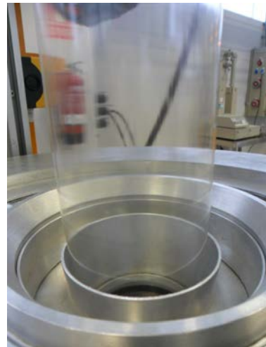
Blow film extrusion
